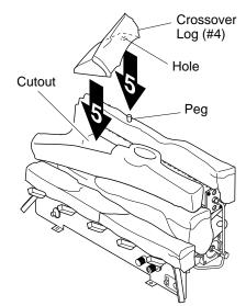
Figure 20 - Installing Crossover Log (#5)
